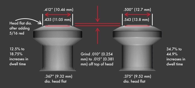
Grind .010 or .015 off head to increase head flat diameter, & standardize working length to the TSM standard +/-.001, or +/-.0005 tolerance to control weight & density.
