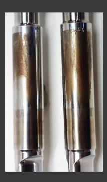
Insufficient Press Lubrication leads to excessive heat and burnishing of tool bodies.
